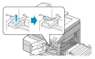
4 Remove the drum cartridge from its bag and slide it into the machine firmly until it locks into place completely.
